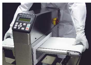
One-touch attachment/ detachment of the conveyor
