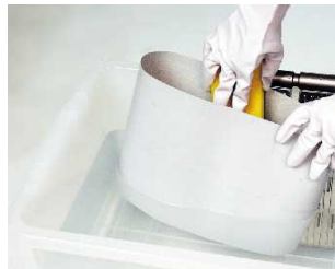
Transfer belt can be cleaned by boiling
